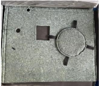
A photograph of a rectangular acoustic enclosure. The enclosure is made of a grey, fibrous material. It has a circular opening on the front face, which is covered by a dark, square-shaped panel. There are also some small holes and a rectangular cutout on the top surface. | Назначение: для снижения уровня шума компрессора. |
